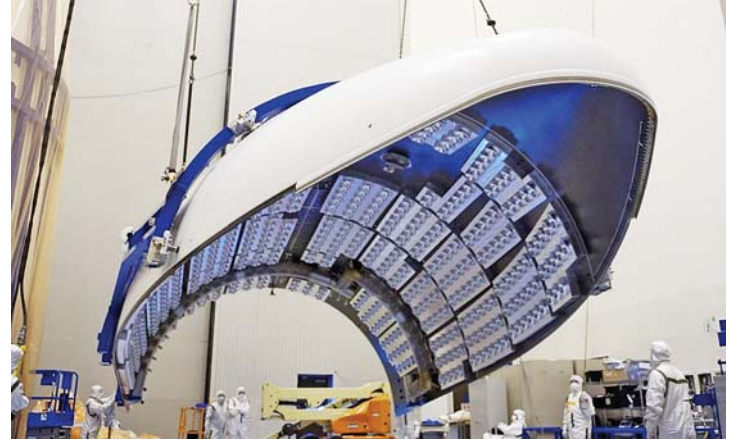
fairing acoustic protection (FAP) system lining the inside of the Atlas V payload fairing
